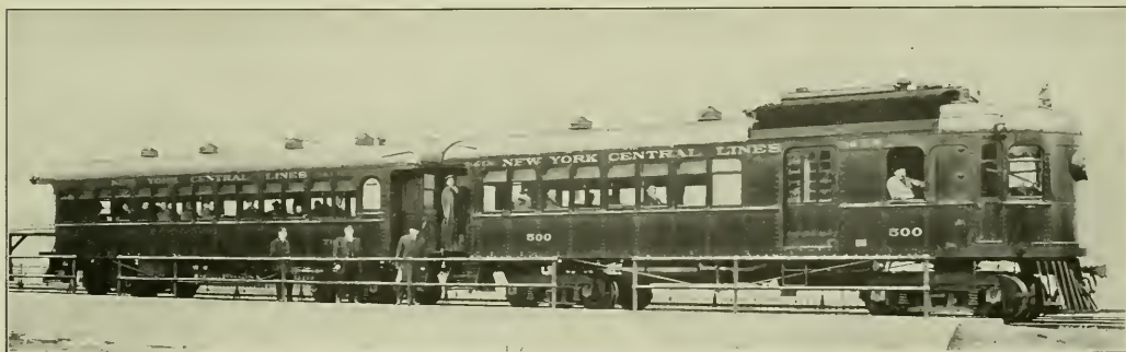
Gas-Electric Motor Car and Trailer Used on the Pittsburgh & Lake Erie.
